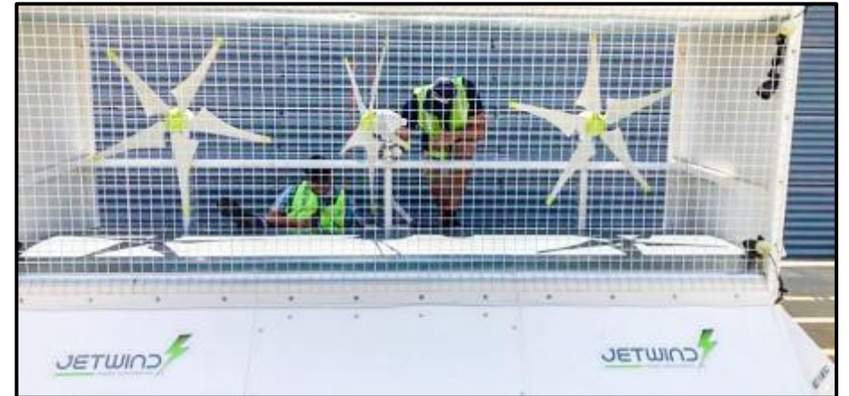
Dallas Love Field: turbine pods convert jet blasts to renewable energy
