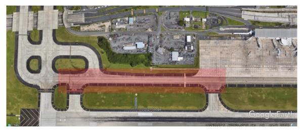
**Scope of the work - Phase 2:** Phase 2 consists of the pavement rehabilitation of Runway 8-26, the primary departure runway at the Airport due to its length, 10,400 feet.
