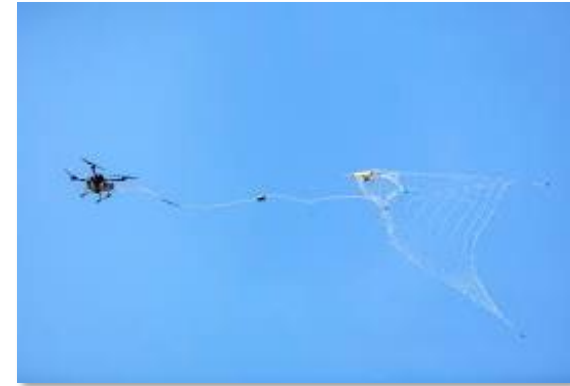
Drone Tracking & Netting System
