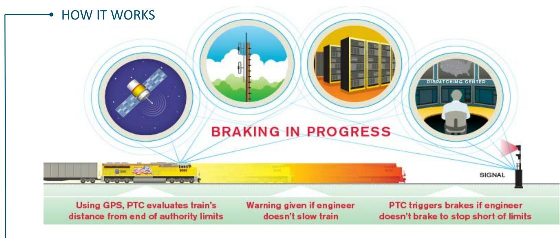
For example, PTC can force a train to stop before it passes a signal displaying a stop indication, or before running through an improperly lined switch, averting a potential collision.
