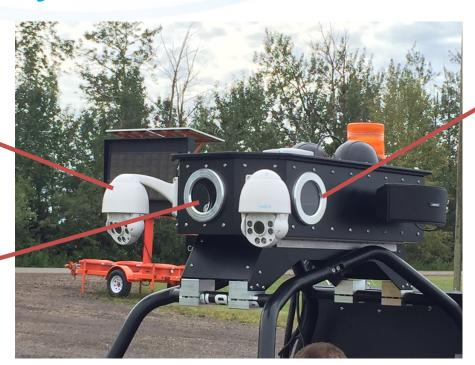
Side cameras for fence integrity check (using artificial intelligence)
